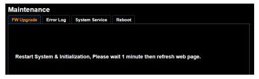
3.6 Please do the [Factory Reset] to ensure the procedure is completed. [Maintenance]-->[System Service]-->[Factory Reset]
